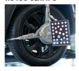
Using optimal force, the clamp attaches to the tire without contacting the rim, providing safe, speedy and uniform clamping operation.
